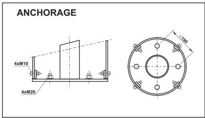
Base -038-**Bolt M10** Nut M20 Washer Flange F100 Last revision: 2007.12.10
