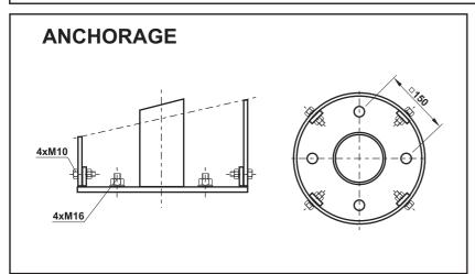
Base -038-**Bolt M10** Nut M16 Washer Flange F100A
